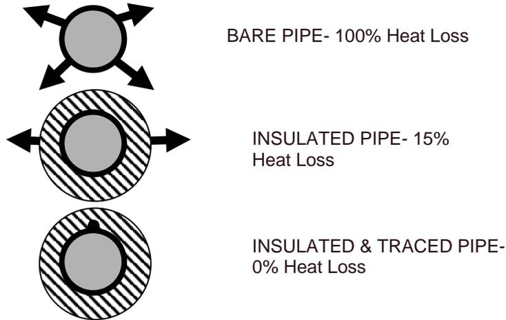
A bare pipe having heated fluid would have a 100% heat loss rate. Whilst a thermally insulated pipe would cut down the heat loss rate by 85%, thus leaving the heat loss rate reduced to 15% only. Replenishing just this 15% heat loss rate by means of a heat tracer, would result in zero heat loss rate from the heated fluid in the pipe.
