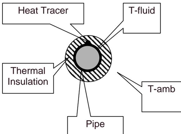
Heat Loss is a function of: a) differential temperature between Pipe fluid temperature and the Ambient temperature; b) outer surface area, which depends on the pipe outer diameter; c) Thermal Insulation thickness; d) Thermal conductivity of Insulation material
